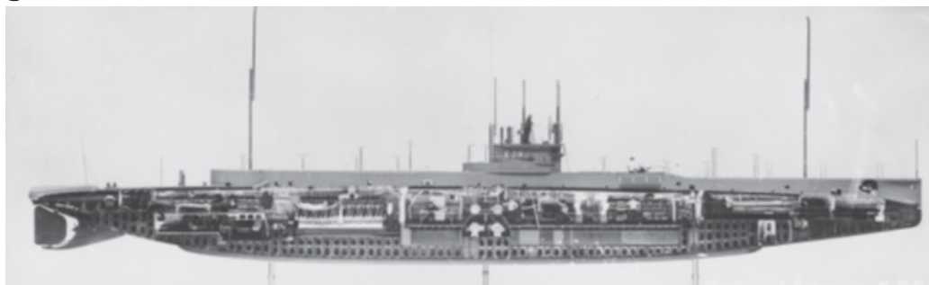
A cut-away model of a British E-class submarine, like the AE2. AWM H12299 These submarines were around 55 metres long and carried a crew of 35. What jobs would the sailors have had to do on board the AE2?
